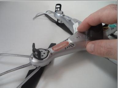
Place one hand on the drone and carefully remove the landing gear with the other hand.
