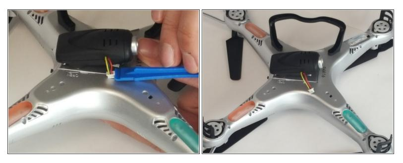
Use the fine edged plastic opening tool to pull up one side of the plug, and then the other, until it comes loose.
