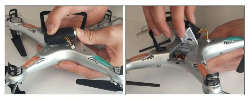
Push the battery cover away from the drone and carefully open it up.
