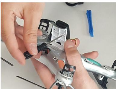
Carefully remove the two Phillips 5.35 mm screws holding the camera to the battery cover.
