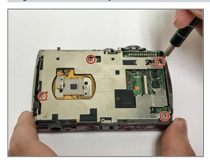
Using a Phillips #000 screwdriver, remove the four 4-mm screws from the metal place.
