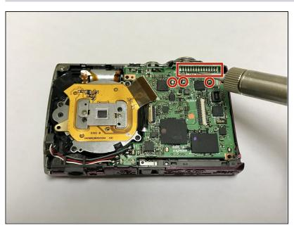
Remove the solder using a soldering iron by following the instructions in this guide.
