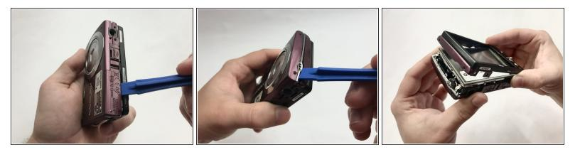
Insert the plastic opening tool into the seam where the front and back parts of the case meet on the bottom of the camera, and slide it along the bottom. Continue along the next side to separate the back part of the case.
