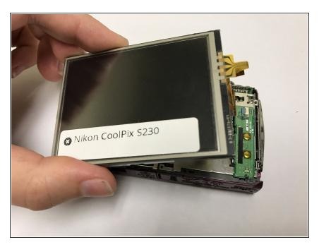
• Lift the LCD screen away from the camera.
