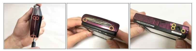
$\bigwedge$  Ensure the camera is turned off and the battery is removed.
