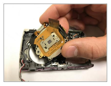
• Lift the lens assembly from the camera.
