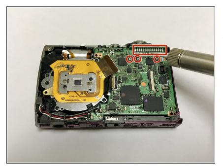
Remove the solder using a soldering iron by following the instructions in <u>this guide</u>.
