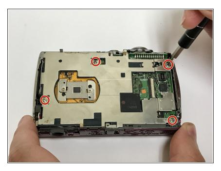
Using a #000 Phillips screwdriver, remove the four 4-mm screws from the metal plate.
