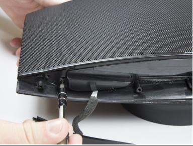
Use a TR 10 screwdriver to remove two of the 10mm screws that secure the speaker grille.
