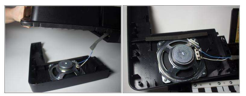
• Gently remove the speaker and its compartment from the front of the keyboard.
