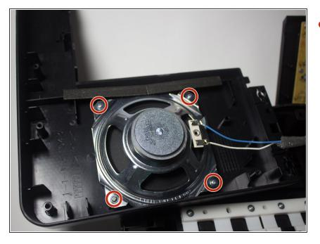
Remove the four 11 mm screws with JIS-1 screwdriver on the four corners of the silver square on the back of the speaker.
