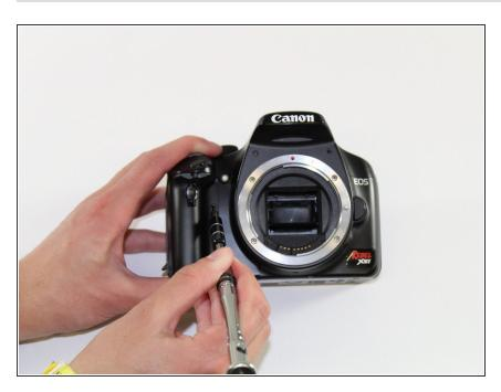
Using the PH000 screwdriver head, unscrew the 3 mm screw that was under the grip
