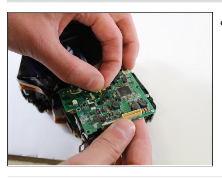
Disconnect cables by pulling out from base with fingers
