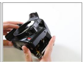
Remove the front panel by using tweezers to pry the panel over the metal ring protrusion
