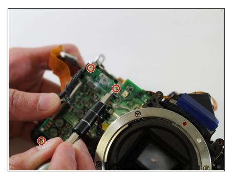
Using the PH000 screwdriver head, remove the three 3mm screws
