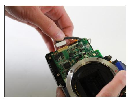
Carefully remove the cable from its plastic base with fingers
