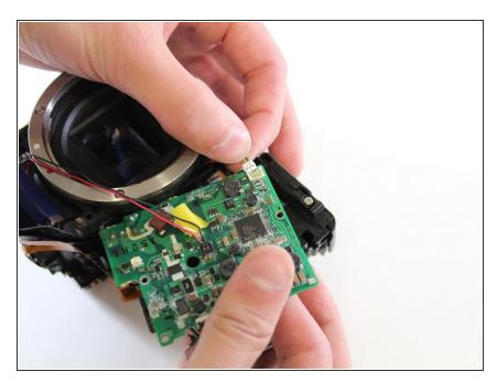
Gently disconnect cable by pulling out from plastic base with fingers
