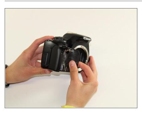
Remove front grip by gently peeling from the edge towards the center of the camera
