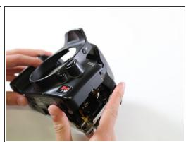
Remove the front panel by using tweezers to pry the panel over the metal ring protrusion
