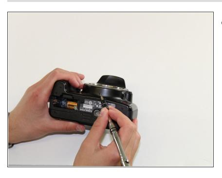
Using the PH000 screwdriver, remove the 4mm screw at the bottom of the camera
