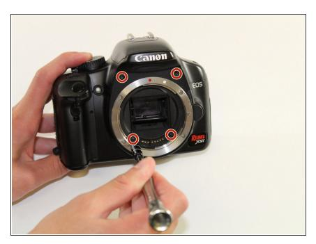
Using the PH000 screwdriver head, remove the four 3mm screws on the front
