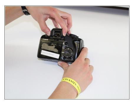
Squeeze the eyepiece between your index finger and thumb and lift up and off.
