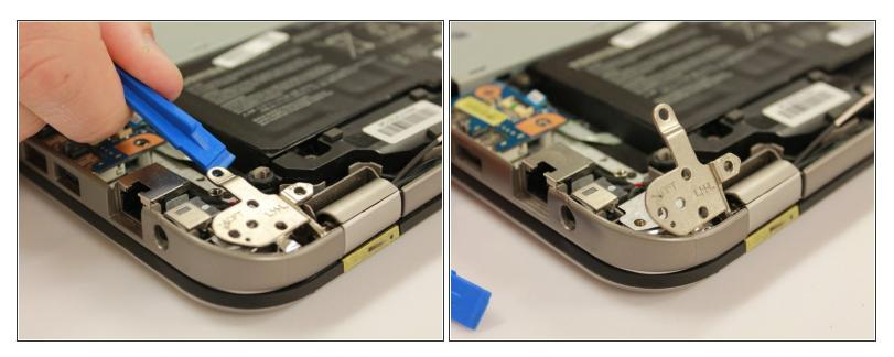
• Use the plastic opening tool to push the left hinge up.
