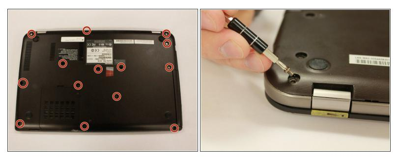
Using the #PH0 screw head, remove 14 (5.7 mm) screws from the back casing.
