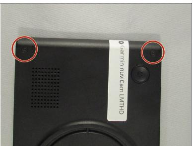
Remove the four 6.9 mm black screws using the T6 screw bit.
