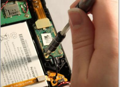
Unscrew six 5.74mm silver screws using the T4 screw bit.
