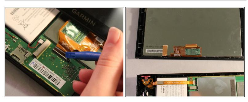
• Disconnect the orange strip by flipping up the connector with a plastic opening tool and sliding the cable out.
