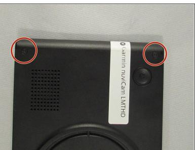
Remove the four 6.9 mm black screws using the T6 screw bit.
