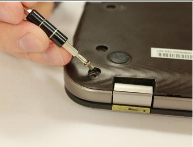
Using the #PH0 screw head, remove 14 (5.7 mm) screws from the back casing.
