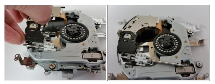
• With the slider's cover plates removed, shift the laser assembly up slightly and out to the left.
