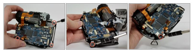
• Remove the three black screws (5 mm, Phillips #00) connecting the frame to the disc housing.
