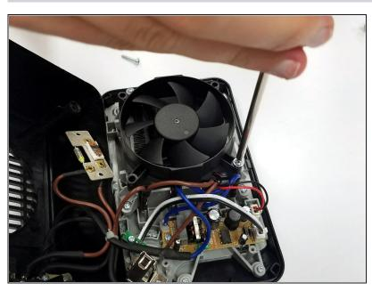
Unscrew the four 9 millimeter, sharp-point screws holding the fan in place.
