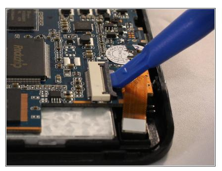
Use the plastic opening tool to open the ZIF connector tab to release the camera's ribbon cable.
