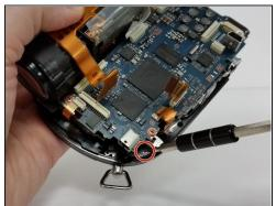
Remove the three black screws (5 mm, Phillips #00) connecting the frame to the disc housing.
