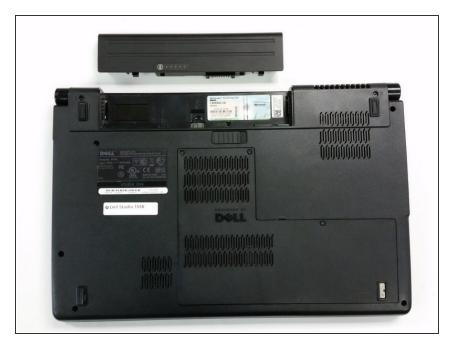
The battery has been successfully removed.
