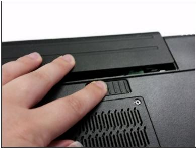
While holding down the slider, gently remove the battery.
