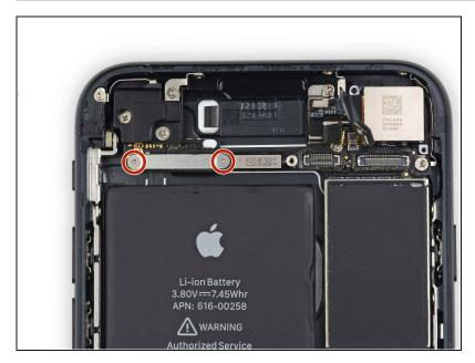
Remove the two 1.2 mm tripoint screws securing the upper cable bracket.
