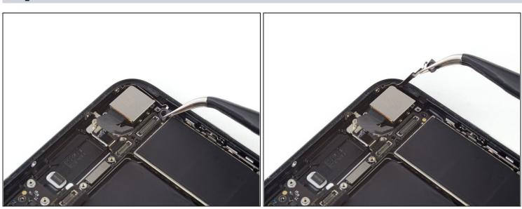
• Use <u>tweezers</u> to gently bend the logic board grounding bracket out of the way.
