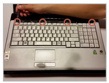
Use a PH0 screwdriver to unscrew the 4 screws at the top of the keyboard.
