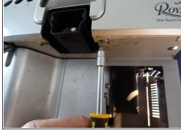
• The screws are situated on the underneath of the cover. This type is held by four screws.
