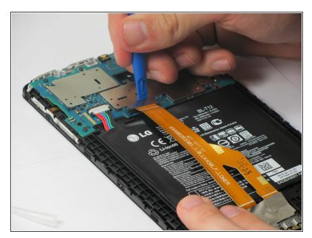
Locate the large orange ribbon cable, pry off the side shown in the image.
