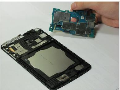
Remove the motherboard by prying it out with the plastic opening tool (as shown in image).
