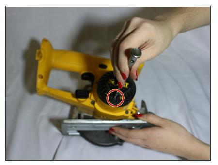
Using a T-20 hex head screw, unscrew the two screws located at the top and bottom of the black air filter. The screws are directly above and below the yellow lettering.
