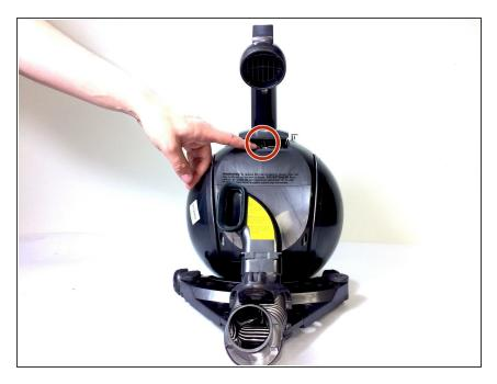
Locate the spring in the small opening between the handle and ball of the vacuum body.
