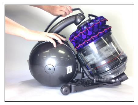
If the top handle does not pop up when trying to remove canister, press the gray button as you gently pull up on the top handle.
