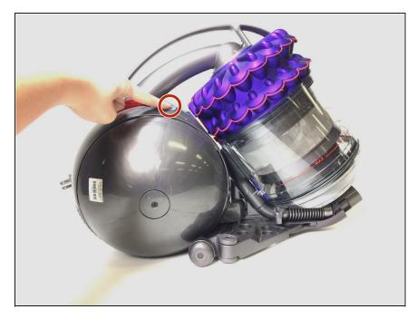
Press the gray button to release the canister.
