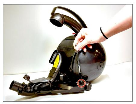
Remove Stabilizer Wheel assembly by removing the 19 mm screw shown in the picture using a T15 Torx bit.
