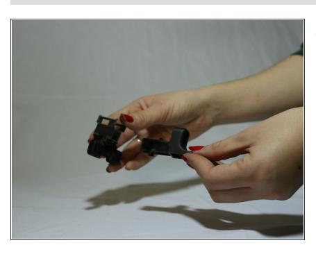
Pull plastic trigger out of the black plastic casing. To reassemble your device, follow these instructions in reverse order.
