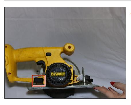
Unscrew the black plastic knob underneath the trigger.
