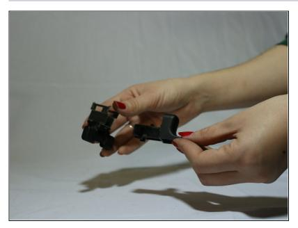
Pull plastic trigger out of the black plastic casing.
