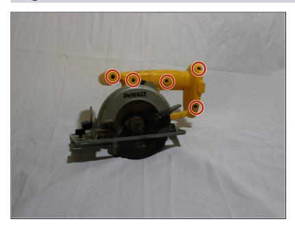
Use a T-15 hexhead screw to unscrew 5 hexagonal screws.
