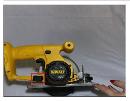
Unscrew the black plastic knob underneath the trigger.
