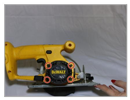
Use a T-20 hexhead screw to unscrew 4 hexagonal screws surrounding the base of the black air filter. The screws are on the yellow portion.
