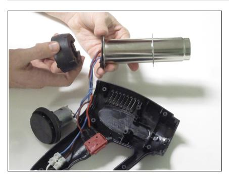
Remove the plastic casing from the end of the barrel.
