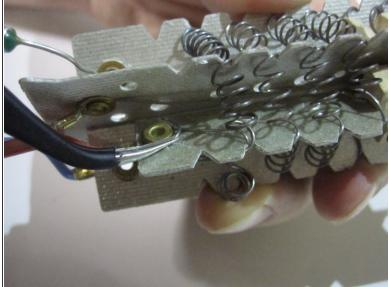
• Use the angled tweezers to remove the heating coil end from the input point.
