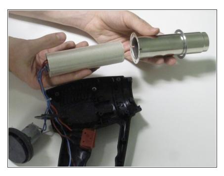
Remove the metal casing from the heating element.
