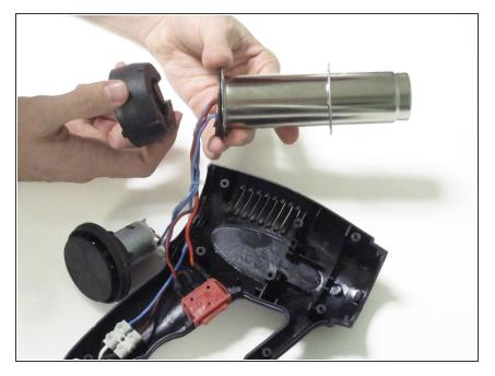
• Remove the metal casing and fan cover from the fan unit.
