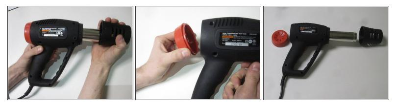
• Remove the barrel casing on either end by twisting and pulling each side off.
