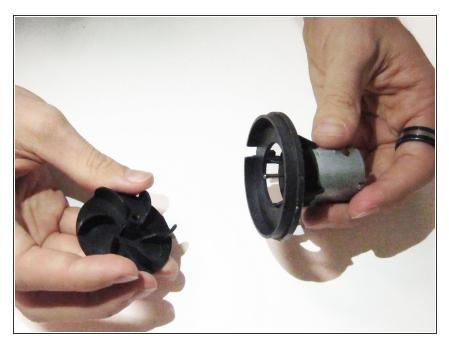
• Remove the fan by pulling it from the motor rod and replace.
