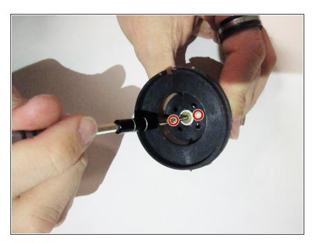
Remove the two 12mm screws from the plastic fan casing using PH#00
