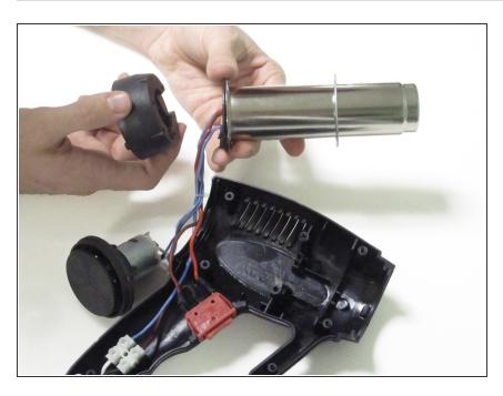
Remove the metal casing and fan cover from the fan unit.
