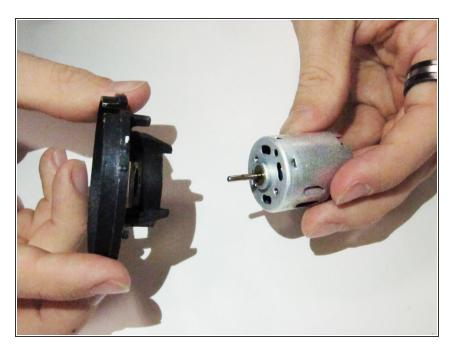
Remove the fan by pulling it from the motor rod.
