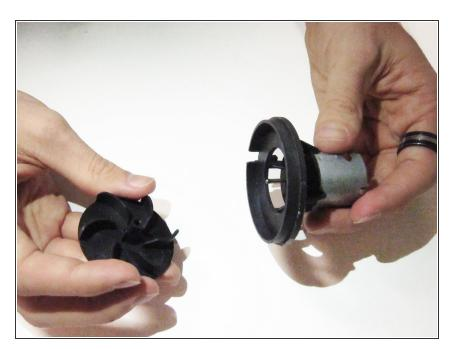
Remove the plastic fan casing.
