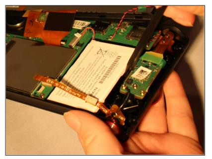
Locate the white box in your device which is the battery.
