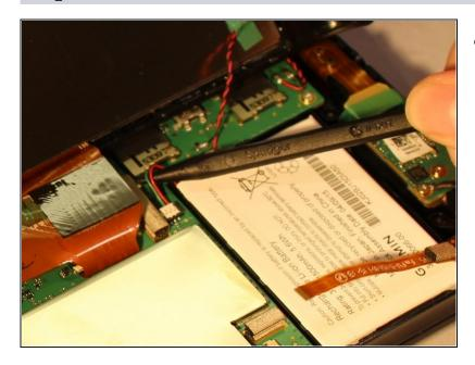
Disconnect battery from device pulling the green, red, and black wires from motherboard.
