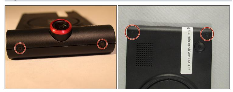
Remove the four 6.9 mm black screws using the T6 screw bit.
