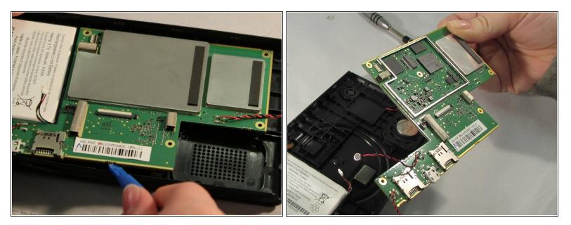
• Lift motherboard out of device using plastic opening tools.
