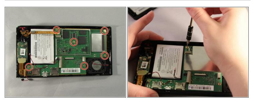
• Remove all six 5.74mm screws from motherboard using the T4 screw bit.
