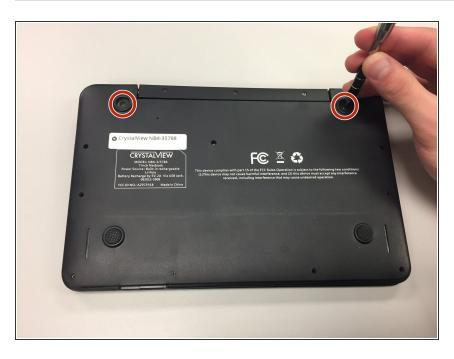
Using a Phillips #00 Screwdriver, remove the screws located under the top two standoffs.
