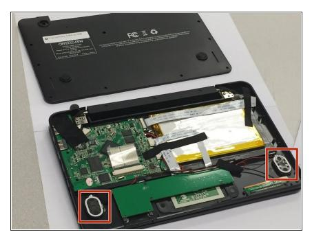
Two speakers can be found on the device, one in the lower-right corner and one in the lower left-corner.
