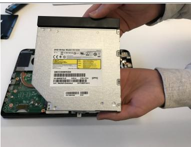
Slide the disc drive to the left. It should come off with ease.
