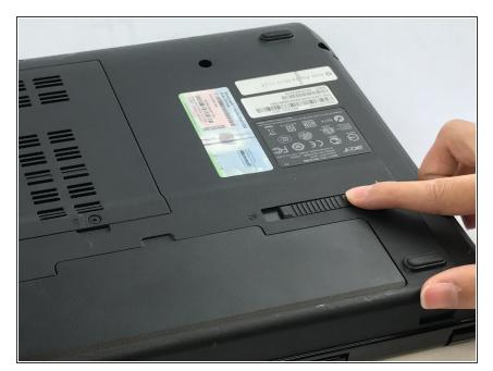
Once unlocked, move the larger switch on the right to the left to release the battery.
