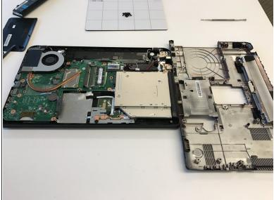
• Using the plastic spudger, pry the back off along the periphery of the laptop.
