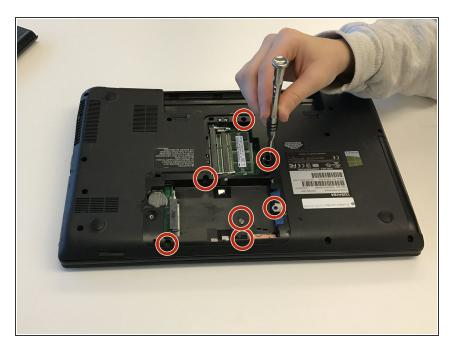
Remove hard drive cover. Using the Phillips Head #0 Screwdriver, remove seven 3mm Phillips #0 screws as indicated.
