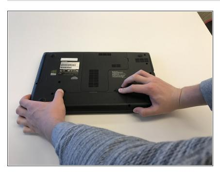
Place fingers on the latches and slide outwards to unlock.
