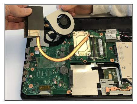
After unscrewing, remove the heatsink from the laptop.
