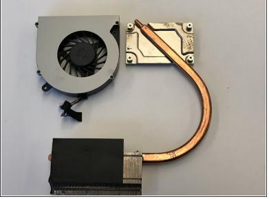
Unplug connected wire to remove the fan as indicated. Both the heatsink and fan should be removed before replacement.
