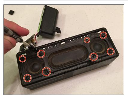
Remove the eight black screws with a Phillips #1 screwdriver.
