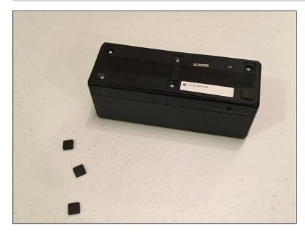
Remove the rubber feet on the bottom of the device.
