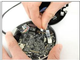
Disconnect the two cables from the camera base motherboard by gently but firmly pulling directly away from their respective ports.
