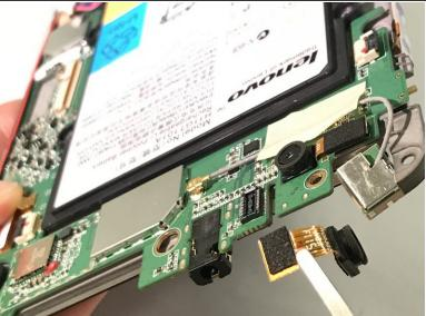
Using the tweezers, pull and remove the front camera component.
