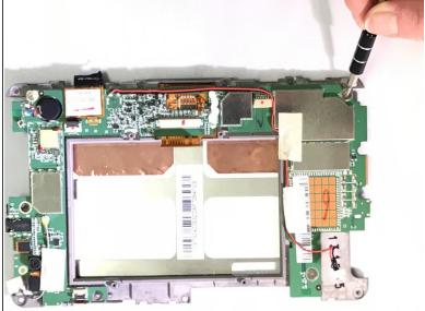
Remove the three screws that are 2.0 mm in length and have a 5.25 mm head width with a Phillips #00 screwdriver.
