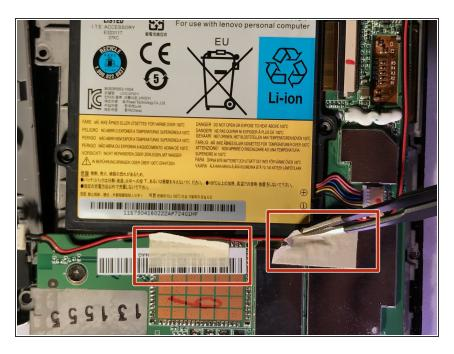
Use tweezers to remove the tape covering the battery's wiring.
