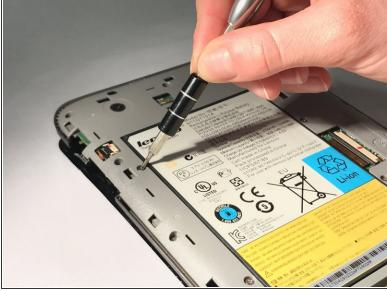
• Use a Phillips #000 screwdriver to remove the seventeen 4mm screws.
