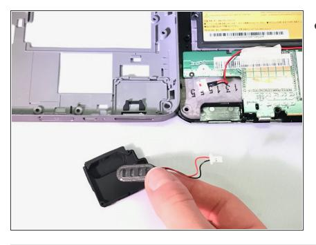
Remove the speaker component from the rubber casing.
