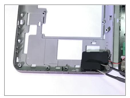
Use tweezers to pull the speaker off of the casing.
