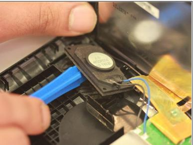
Use the plastic opening tool to pry the speaker away from the device.
