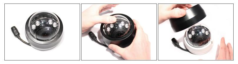
• Lift off the paintable snap-on cover from the AvertX HD810 dome security camera.
