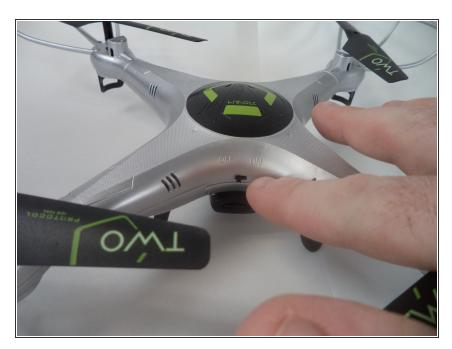
Turn device off by moving the selector switch to the left.
