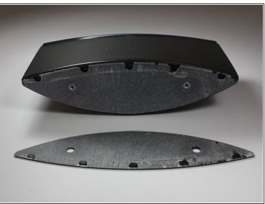
Use a spudger or your fingers to pry off and remove the rubber pad on the bottom of the speaker.
