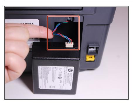
Locate the blue/green/red wire attached to the back of the adapter.
