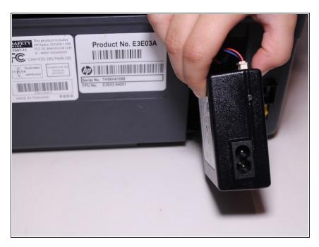
• Remove the HP AC Power Adapter from the slot.
