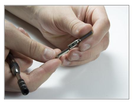
Use a 5 mm hex driver to extend the TR 10 driver. This allows the driver to access screws with deeper countersinks.
