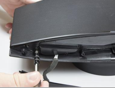
Use a TR 10 screwdriver to remove two of the 10mm screws that secure the speaker grille.
