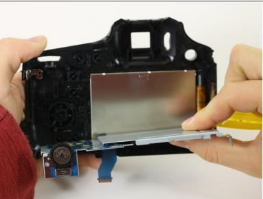
Remove the entire silver panel to reveal the back of the LCD screen
