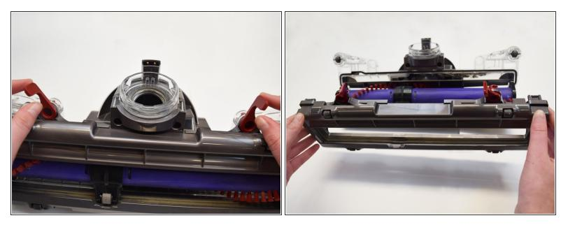
• Lift up on both of the red levers on either side to remove the rectangular dark grey piece that the levers are connected to from the head piece.
