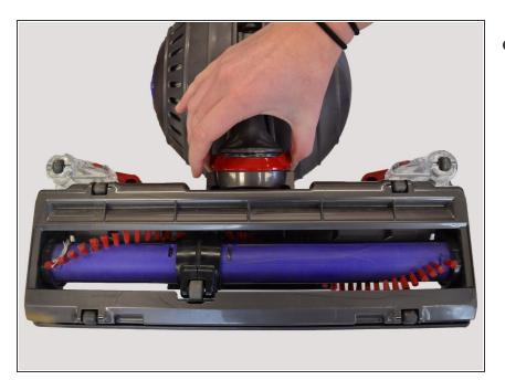
Lay the vacuum on its back and remove the red clip from the bottom front of the vacuum by placing both your thumbs on either side and pulling up.
