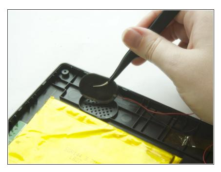
Use the tweezers to lift the speakers out of its compartment, including the felt cover attached to the plastic.
